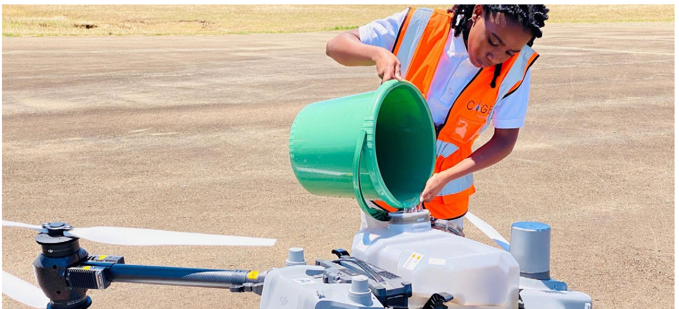
One of the testing team re-filling the The DJI Agras T50 iwhich is capable of carrying 40kg/ ltrs for spraying
